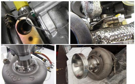
Examples of incorrect sealing wiring
